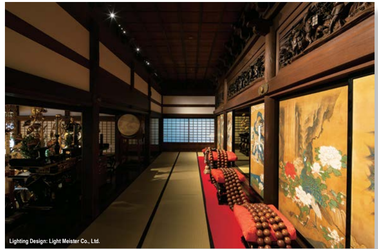
Micro Light Cannon fixtures with 3000K LEDs and a 24 degree lens illuminate this wall.
